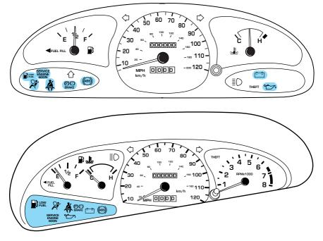
Make sure the corresponding lights illuminate briefly. If a light fails to illuminate, have the vehicle serviced.
